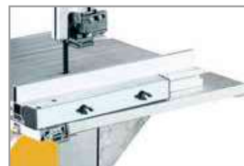
Tilting table up to 45°, goniometer included
