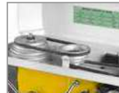
Upper cover opening with safety microswitch Tapa superior con micro-interruptor de seguridad
