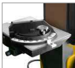
Sander in vertical position with workbench and goniometer
